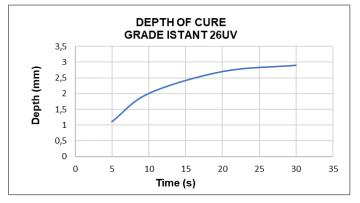
\*Depth of cure depends on the power of the UV lamp, on the emission spectre and on the distance between the lamp and the joint.
